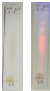
Figure 1 Thin Layer Chromatography (TLC) Results of T. mantaly Stem Ethanol Extract under UV 365 nm Light
